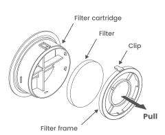
Insert the filter into the back of the filter cartridge, with the firmer side facing the room
