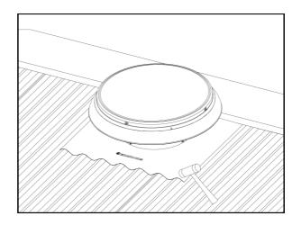
Lift the flashing and run a bead of silicone along the underside of the flashing, following the edge along the three exposed sides.
