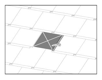
Taking the Airomatic unit slide the flashing under the tiles above the opening.
