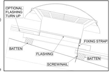
Position the vent in an appropriate position and slip the top edge of the flashing under the ridge capping. Mark the centre of each side to determine where the centre of the vent will be.
